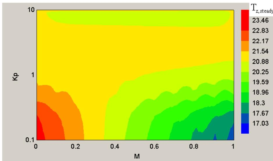
Figure 11 – Effect of gain and bias on the zone steady temperature for the proportional controller case considered.
