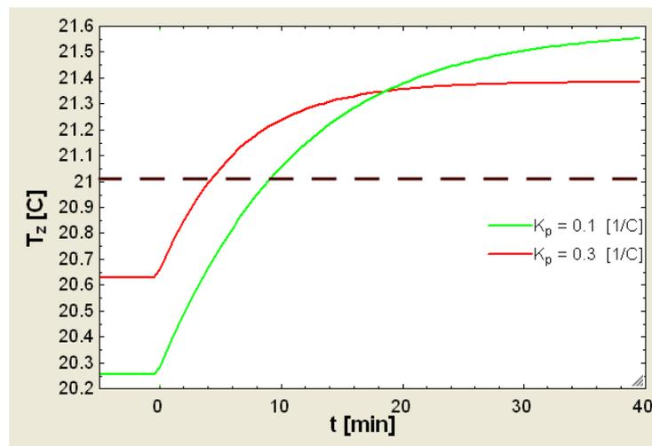
Figure 8 - Effect of gain on the zone temperature response for a proportional control
