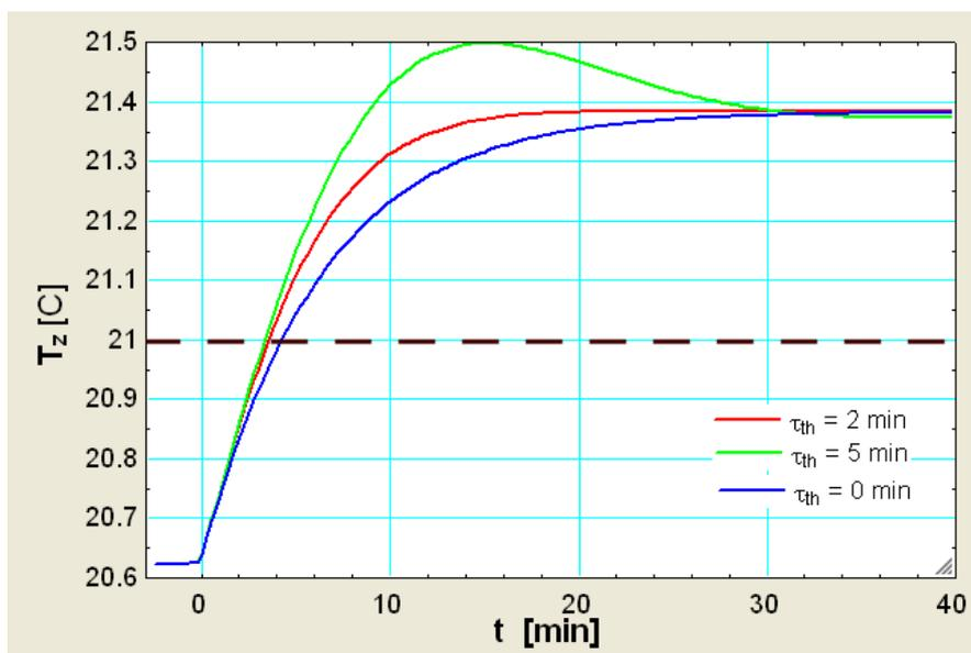
Figure 10 – Thermostat inertia effect on the zone temperature response for a proportional control
