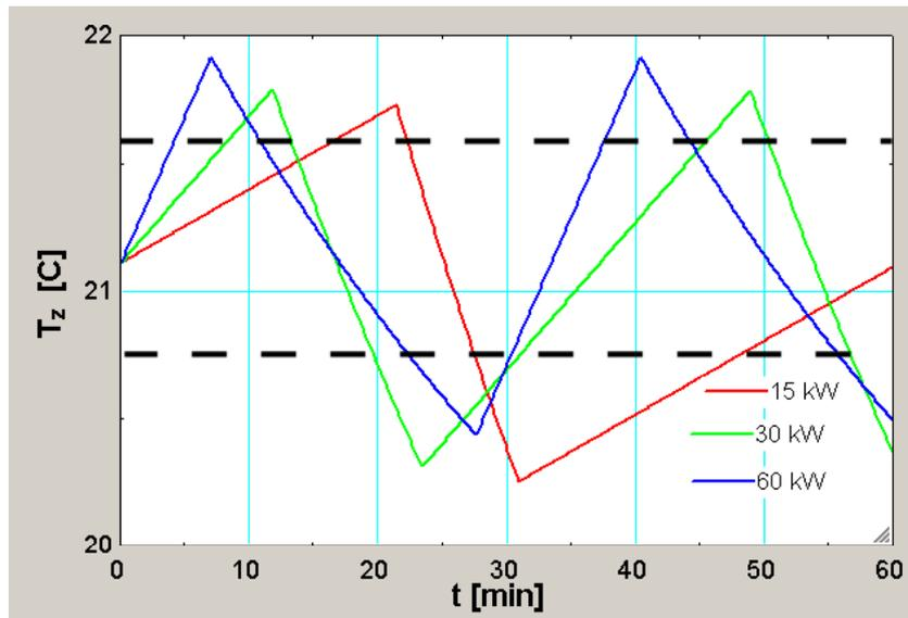
Figure 6 – Effect of zone sensible load on the zone temperature response for an On-Off control
