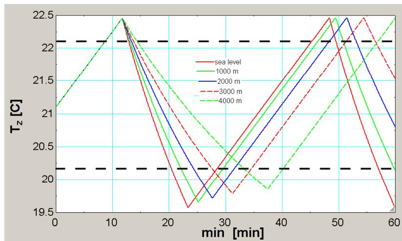
Figure 4 - Effect of altitude on the zone temperature response for an On-Off control
