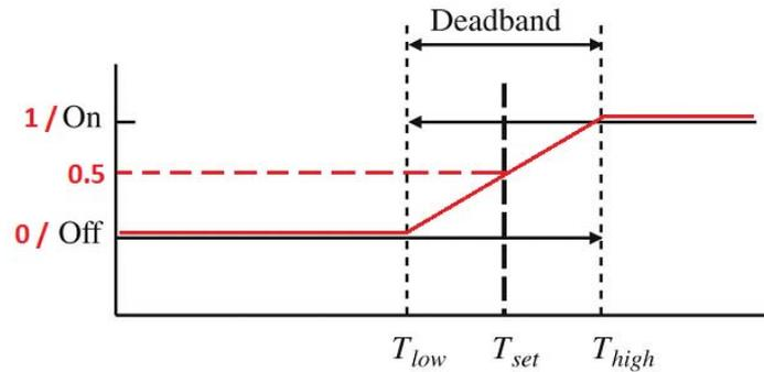
Figure 2. On-Off and Proportional control schemes (adapted from Mitchell and Braun, 2013)
