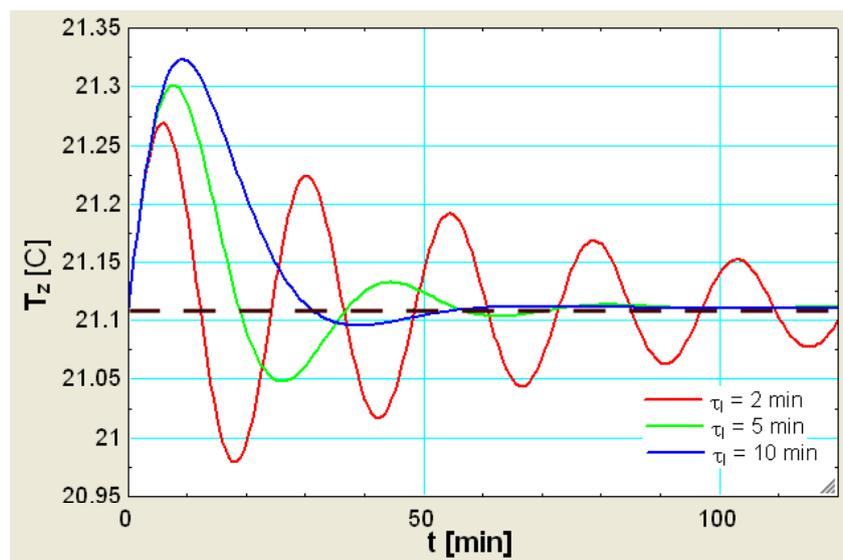
Figure 12 – Effect of integral time constant on the zone steady temperature for a proportional integral controller.
