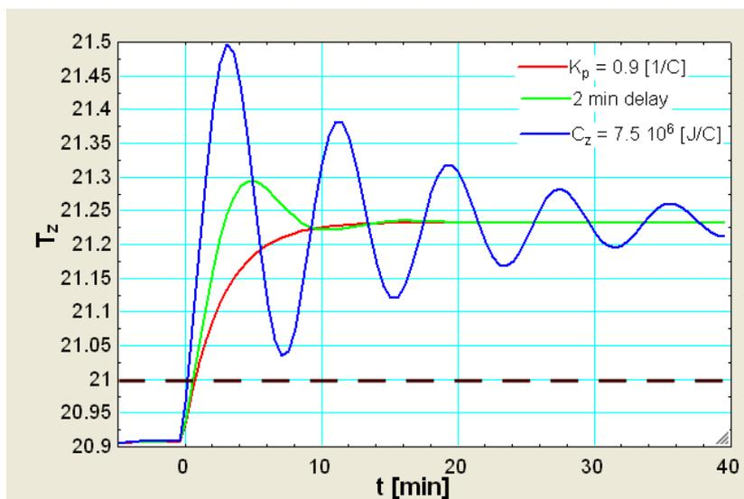
Figure 9 – Cumulative effect of high gain, time delay and low capacitance on the zone temperature response for a proportional control
