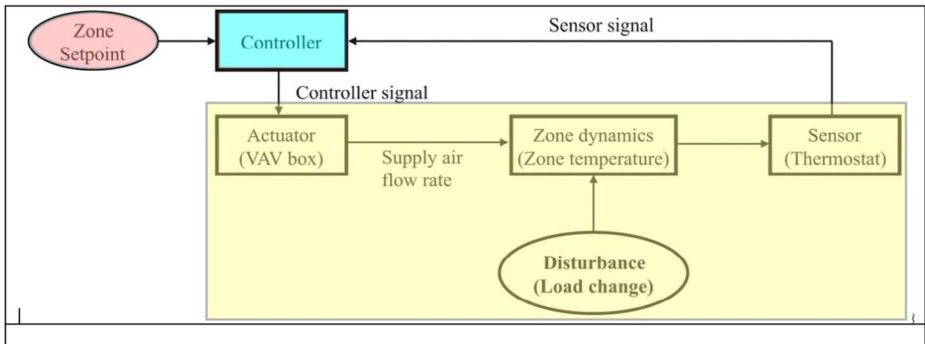
Figure 1 - Block diagram of the control loop (adapted from Mitchell and Braun, 2013)
