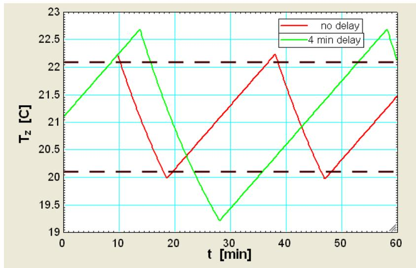
Figure 3. Effect of control action delay on the zone temperature response for an On-Off control
