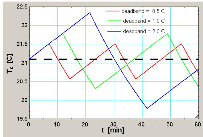
Figure 7 - Effect of deadband on the zone temperature response for an On-Off control
