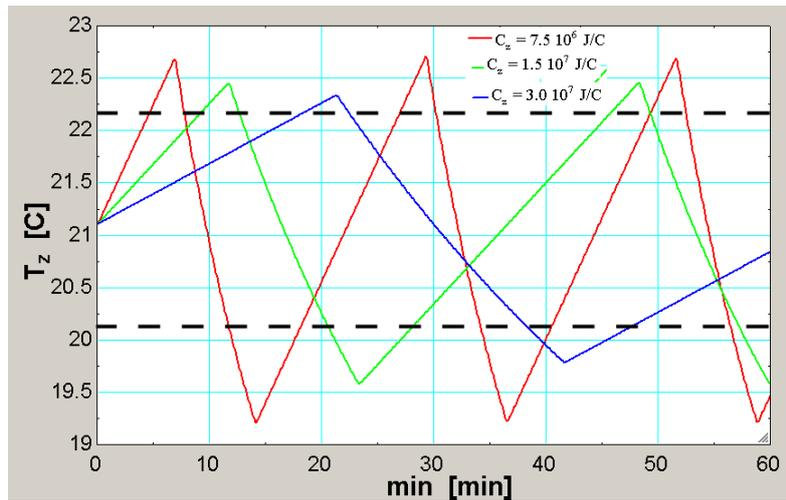
Figure 5 – Effect of zone capacitance on the zone temperature response for an On-Off control
